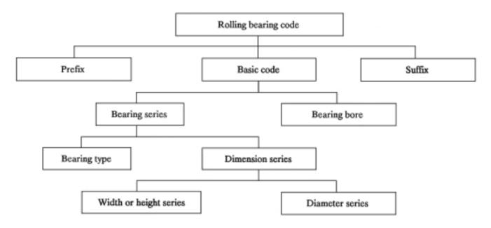
Structure of the rolling bearing code: DIN 623
