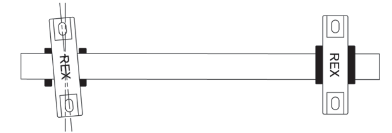
Bolts on Left Bearing are Vertically Misaligned
