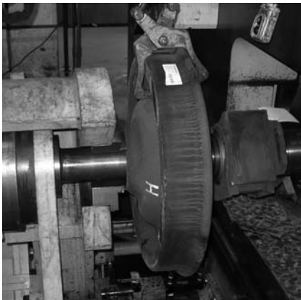
Figure 12 – Wheel being applied with a wheel press.
