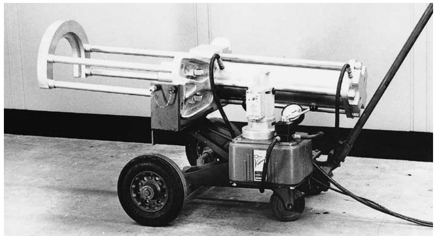
Figure 8 – A self-contained portable machine equipped with a pump for installing and removing bearings.
