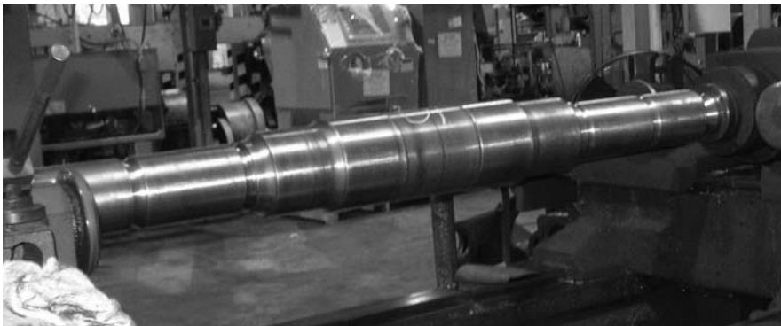
Figure 14 – Axle mounted in axle lathe for inspection.
